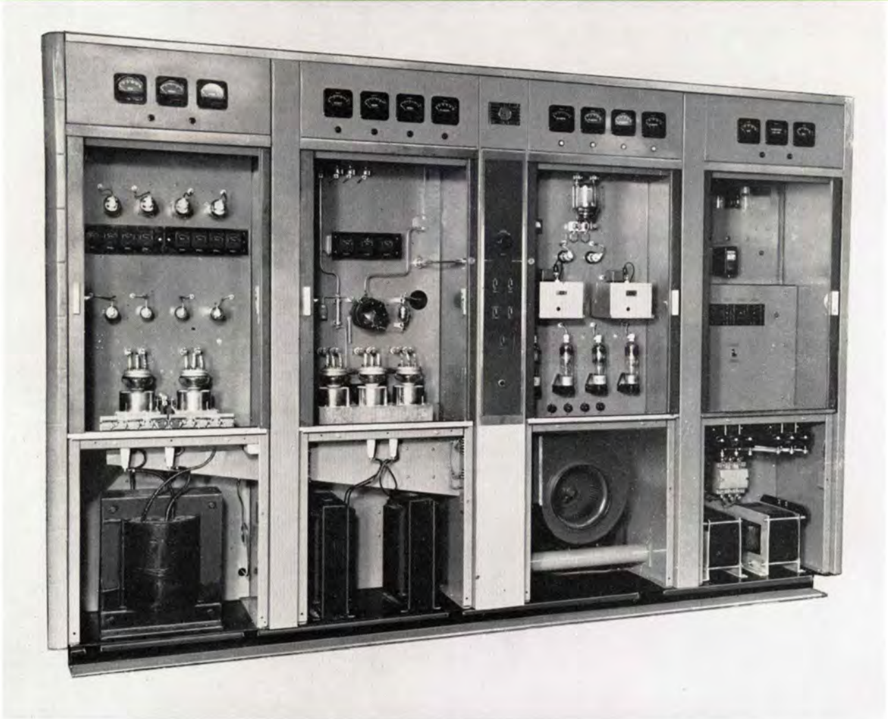
Front view with sliding doors opened and lower panels removed to show interior arrangement. Note the similarity of mechanical layout. Cabinets from left to right house modulator, power amplifier, exciter, and rectifier and control units respectively.
