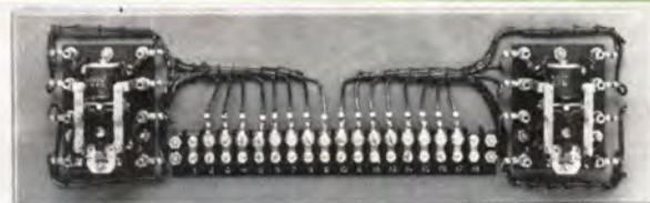
Latching Relay Panel, MI-27509-A.
