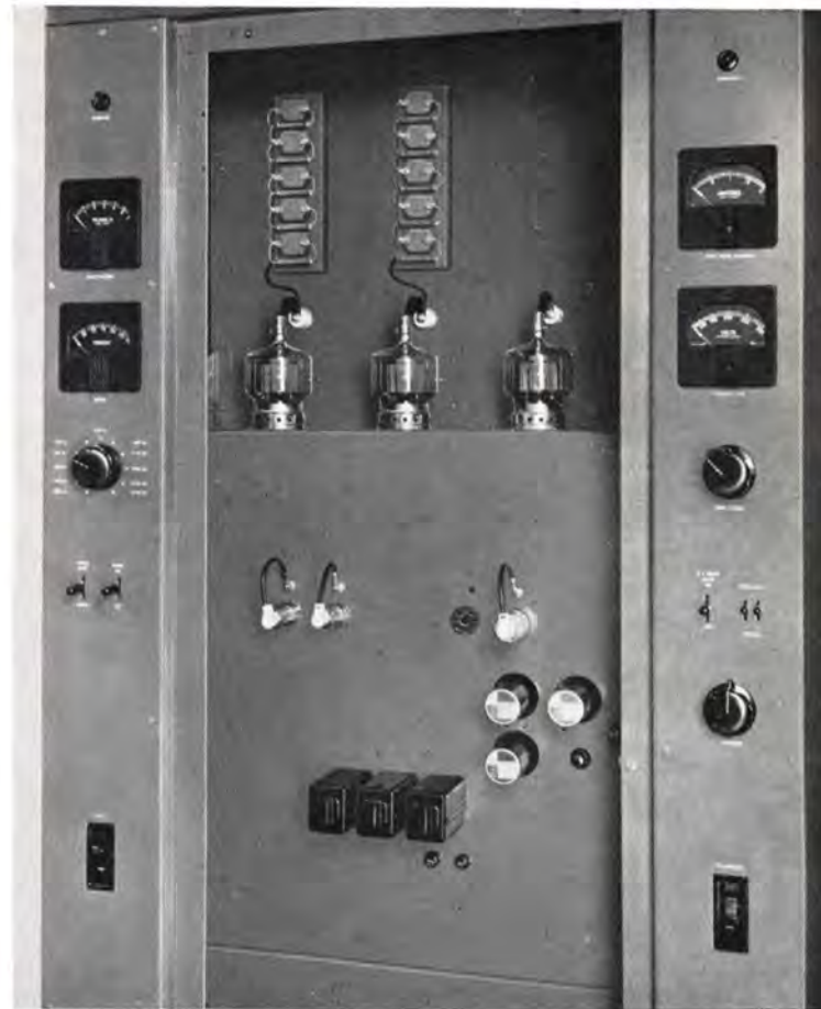
The front of the BTA-500R permits easy tube changes. The power amplifier and modulator tubes are located on the top chassis and just below this is the exciter chassis. All normal operating controls are shown on the two side panels.
