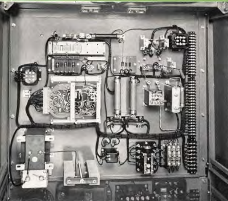
Rear view of entire oscillator subassembly showing vertical construction, plug-in terminal strip, etched wiring and simplified circuitry of BTA-500R AM Broadcast Transmitter.
