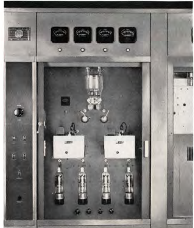
Close up front view of the R-F Driver or Exciter cabinet. Sliding door is fully opened to show tubes, controls and components. Vertical chassis construction is employed throughout the BTA-5H and BTA-10H Transmitters.
