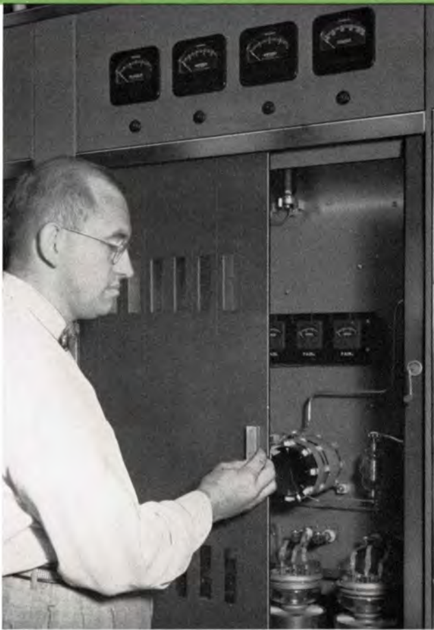
Complete accessibility to all "vertical-chassis" components and tubes is facilitated by the use of horizontally-sliding doors made of extruded aluminum slats. Doors slide back effortlessly on rubber caster assemblies.
